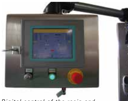
Digital control of the resin and curing agents
