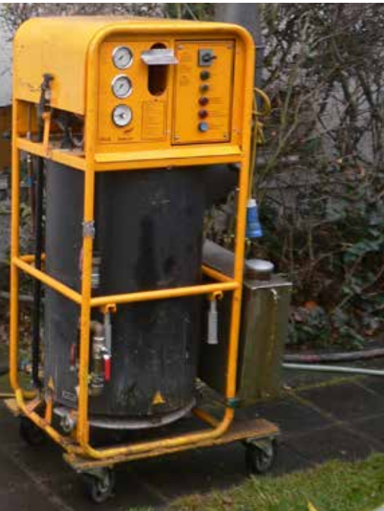
Mobile water heater for rehabilitation lines difficult to access
