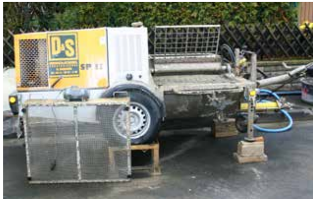
Mortar pump for the operation of the centrifugal engine
